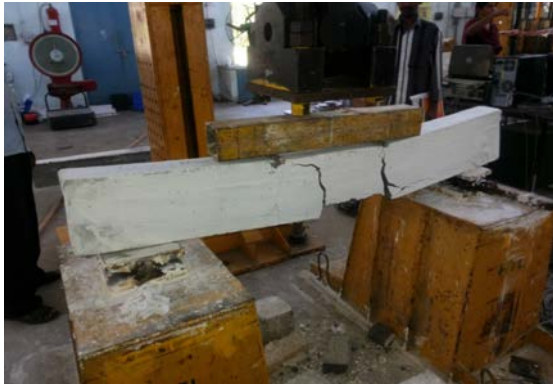
Fig 7: Failure of Basalt Bar Reinforced Concrete Beam
