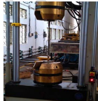
Fig 1: Tension Test on BFRP Bars
