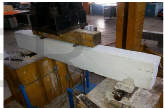
Fig 5: Failure of Steel Reinforced Concrete Beam
